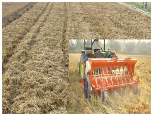
Fig. 2: Happy seeder sowing wheat into rice residue (8.5 t ha<sup>-1</sup>) after uniform distribution of residue
