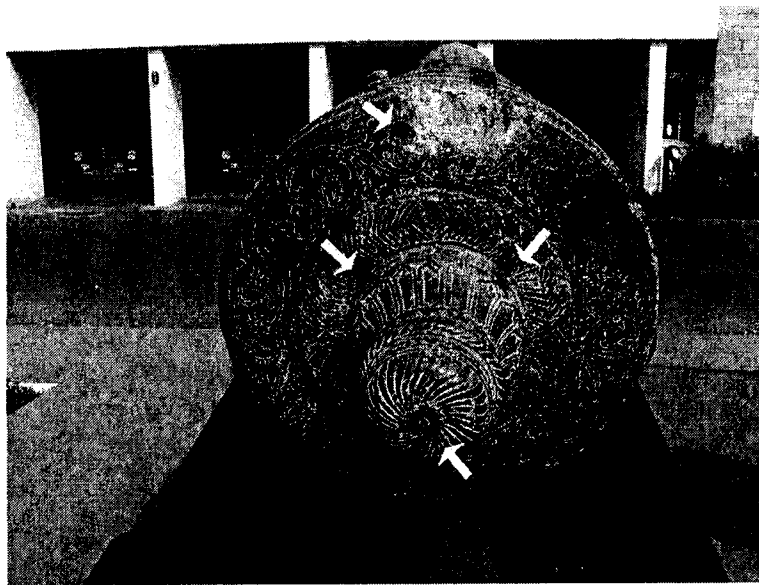
Fig. 9: Rear portion of Zafarbaksh showing the arrangement of iron chaplets (arrowed) in this portion. The intricate design on the rear section also deserves notice.
