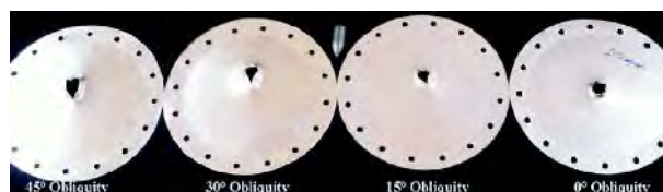
Fig. 9: Deformed specimens of 1 mm thick 1100-H12 aluminum target impacted at different obliquity [6]
