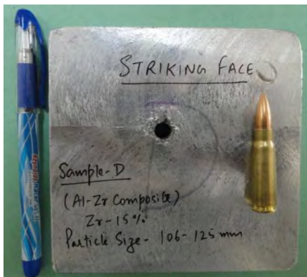
Fig. 6: Ballistic Impact of AK-47 bullet on an aluminium target
